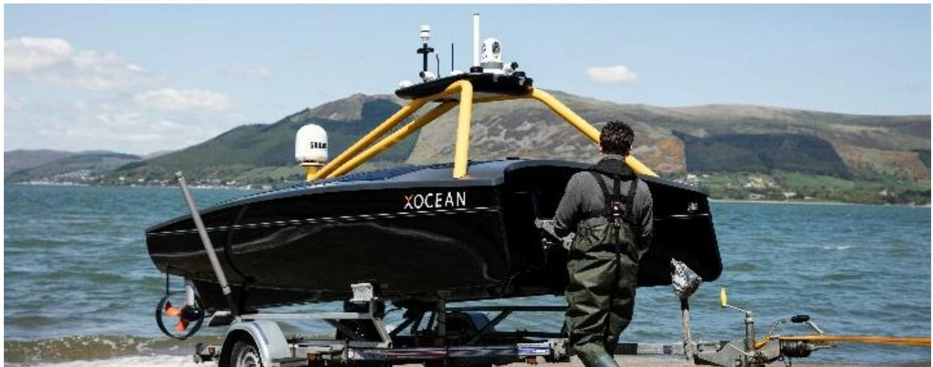
FIGURE 2: XO-450 USV BEING PREPARED FOR LAUNCH
