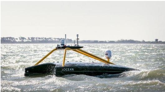
During August, XOCEAN completed a survey of a buried pipeline in the Gulf of Mexico, mobilising out of Port Arthur, Texas. Operating 24/7, XOCEAN's XO-450 completed the mission in 3.5 days using multibeam, sub bottom and magnetometer.
