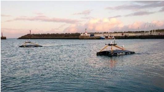
In June, XOCEAN completed a wide area bathymetric survey in the eastern Irish Sea. Multiple USVs were used to complete the 422km<sup>2</sup> survey in depths ranging from 10m to 30m. Survey activity was carried out in a variety of conditions up to Sea State 5.
